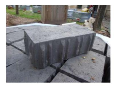
PERMEABLE PAVERS MIN. 3 1/8" (80mm) THICK
